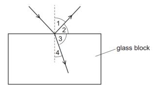
The ray of light is partially reflected back into the air and partially refracted into the glass block.
